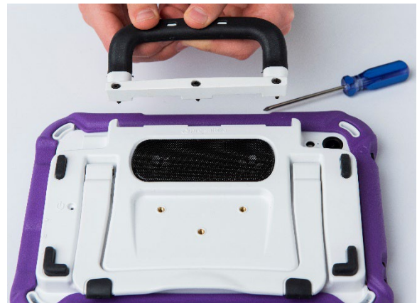
Via Mini: Remove three screws
