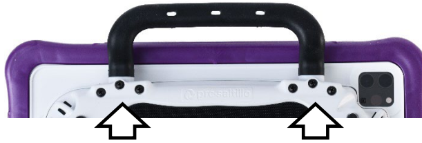
Via Pro: Remove six screws
